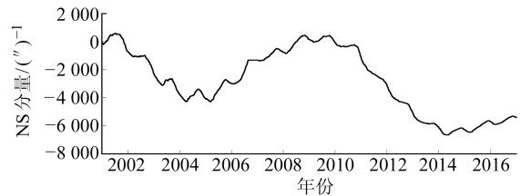
图 1 库尔勒水平摆倾斜仪 NS 分量日值曲线 Fig. 1 The curve of daily observation of Korla horizontal pendulum tiltmeter
